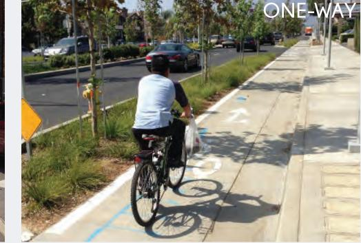
A CYCLE TRACK IS AN EXCLUSIVE BIKE FACILITY THAT COMBINES THE USER EXPERIENCE OF A SEPARATED PATH WITH THE ON-STREET INFRASTRUCTURE OF A CONVENTIONAL BIKE LANE. A CYCLE TRACK IS PHYSICALLY SEPARATED FROM MOTOR TRAFFIC AND DISTINCT FROM THE SIDEWALK (NACTO).
