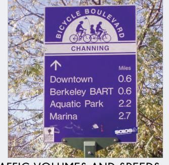
BICYCLE BOULEVARDS ARE STREETS WITH LOW MOTORIZED TRAFFIC VOLUMES AND SPEEDS DESIGNATED AND DESIGNED TO GIVE BICYCLE TRAVEL PRIORITY. BICYCLE BOULEVARDS USE SIGNS, PAVEMENT MARKINGS, AND SPEED AND VOLUME MANAGEMENT MEASURES TO DISCOURAGE THROUGH TRIPS BY MOTOR VEHICLES AND CREATE SAFE, CONVENIENT BICYCLE CROSSINGS OF BUSY ARTERIAL STREETS (NACTO).
