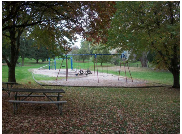
Playground – no accessible route – wood prohibits access
