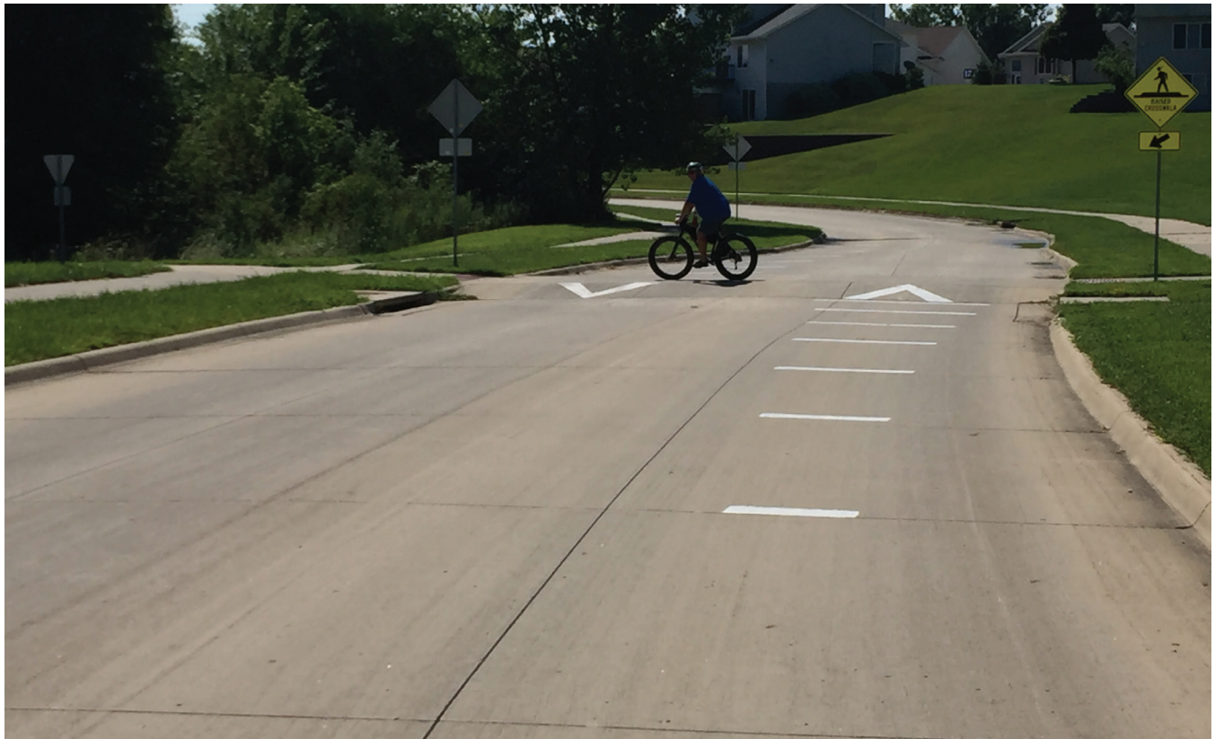
Figure 20. The raised crosswalk and speed humps along Shannon Drive calm traffic and increase safety for bicyclists.
