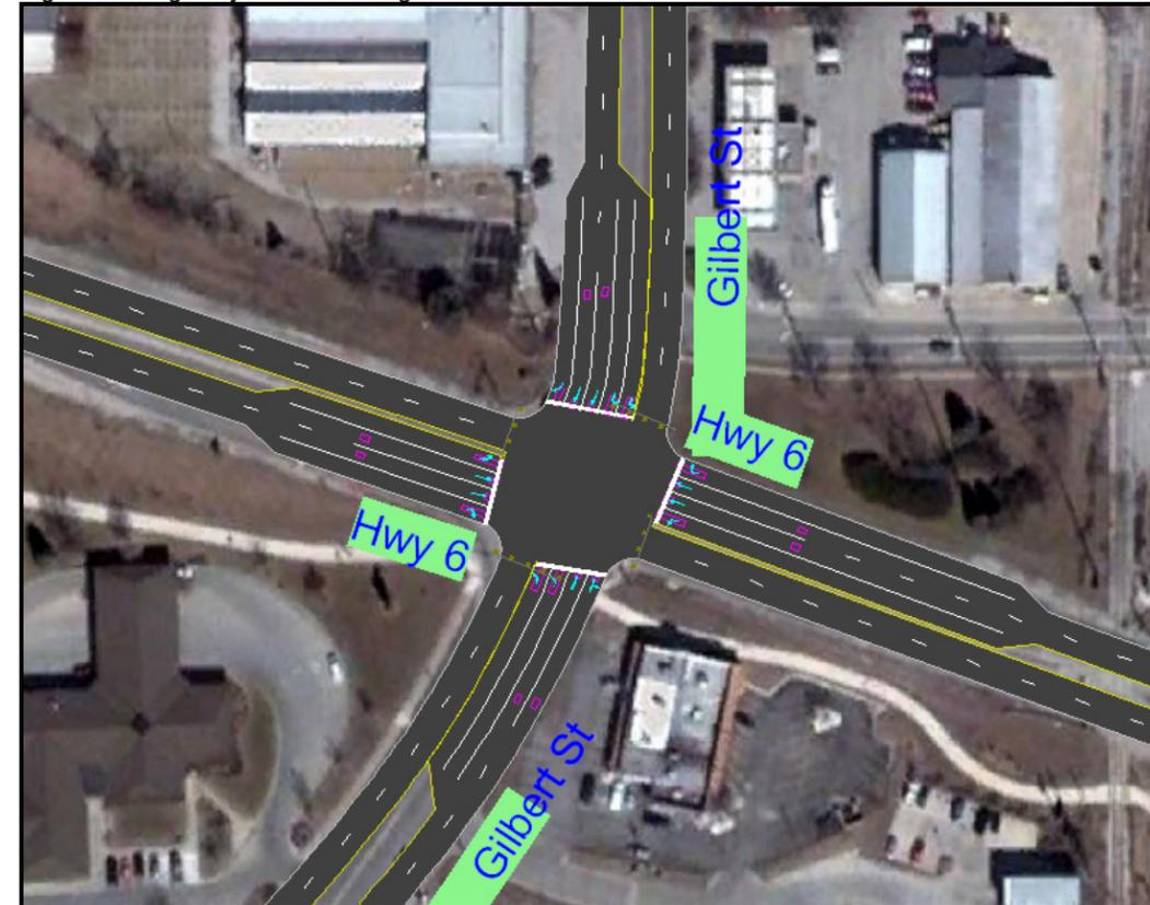
SUDAS Minimum Criteria: For the Highway 6 area, all lane widths should be 12 feet.
