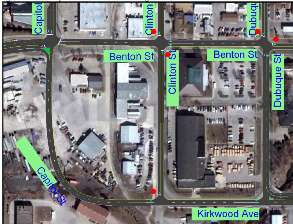
SUDAS Minimum Criteria: For the one-way concept, all lane widths should be 12 feet except:
